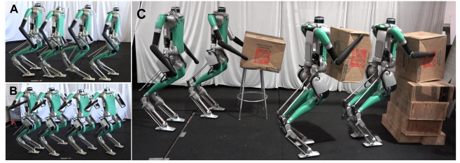
Fig. 2: Real-world demonstrations of our approach. A) Locomotion Directives using joystick commands. B) Fully-specified directive for a boxing jab; showing whole-body torso motion and foot coordination. C) Handcrafted sequence of masked directives combining upper body motion trajectory and lower body joystick commands; showing the ability to move to a location, pick up a box, move while holding it, and place it at a target location.
